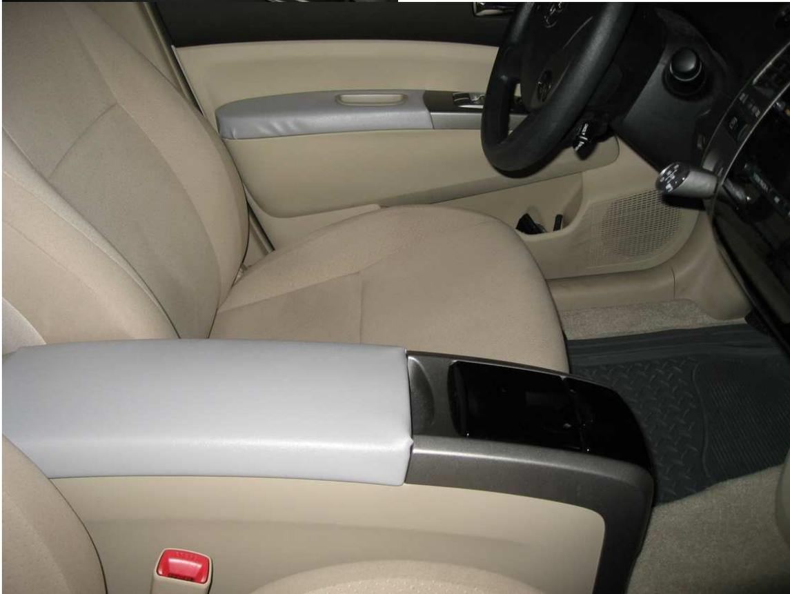
NB: The central armrest is much easier to cover : remove 6 screws and 2 clips, fold it with vinyl and you're done !
