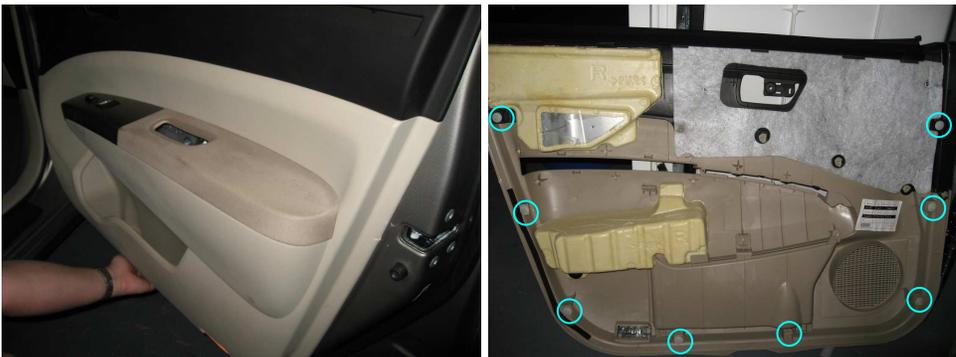
There is a wire connecting the door bulb that you need to remove **before** lifting the door:
