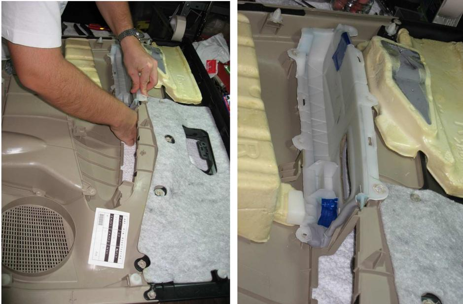
Now we will secure it with screws, since the mounting holes for the screws are not very tall (except one), I took some small wood screws and cut the ends (except one):
