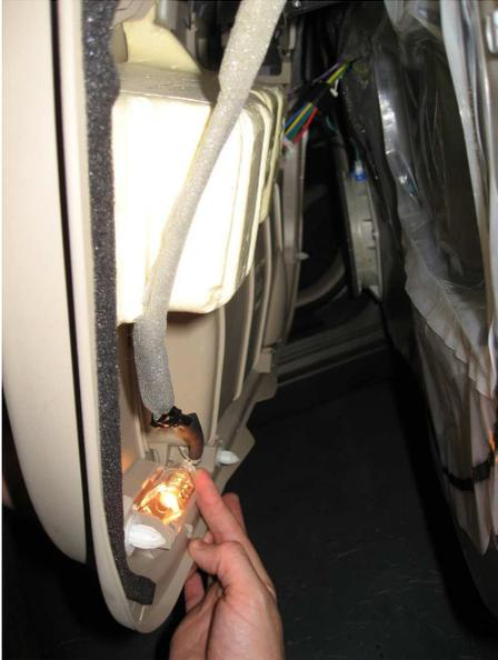
6. Remove the clips that could be stuck on the door and place them back on the door interior
