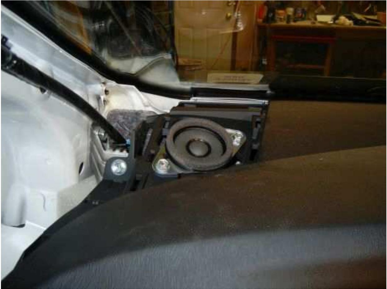
Pull the speakers and disconnect the wiring. The connector has a keeper (on one side) that you depress to release.
