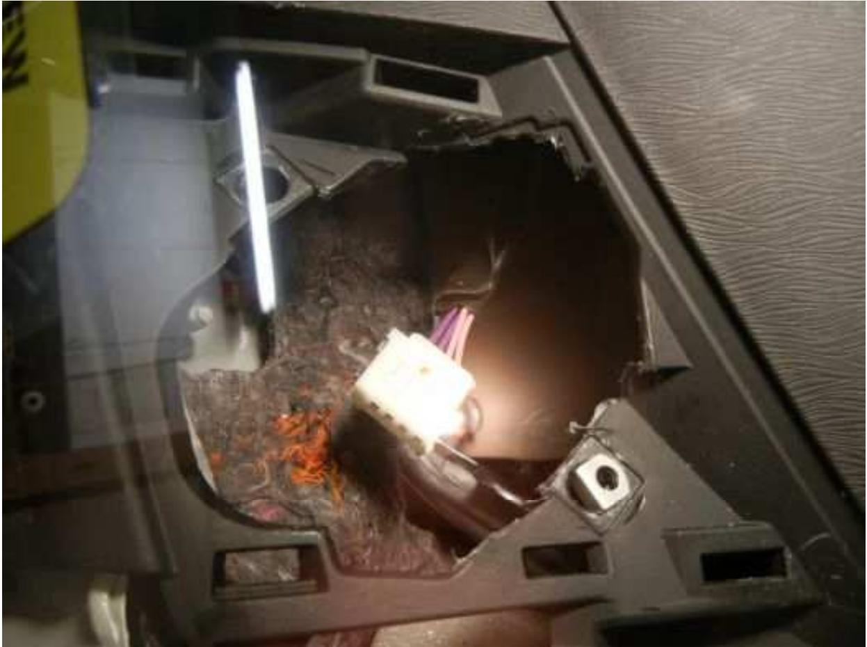
With the speaker is in position, drill hole(s) if necessary. I was able to use one existing hole but had to drill a new one at the top. Drill in the sense I had to use a stubby screwdriver and a self-tapping screw because the windshield obstructs access. \* Be sure not to obstruct the slots where the grill attaches.
