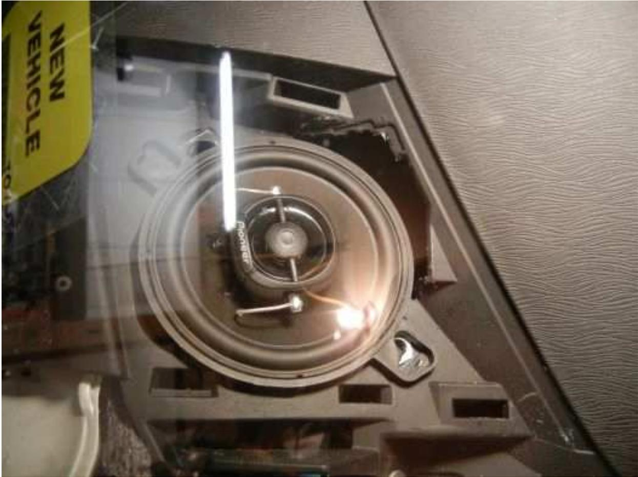
The speaker grills had to be modified. There is a lip that comes down from the bottom side that contacted the new speakers. I used a Dremel to trim this plastic off flush with the grill. In the picture below the grill at the right has been trimmed, the left not.
