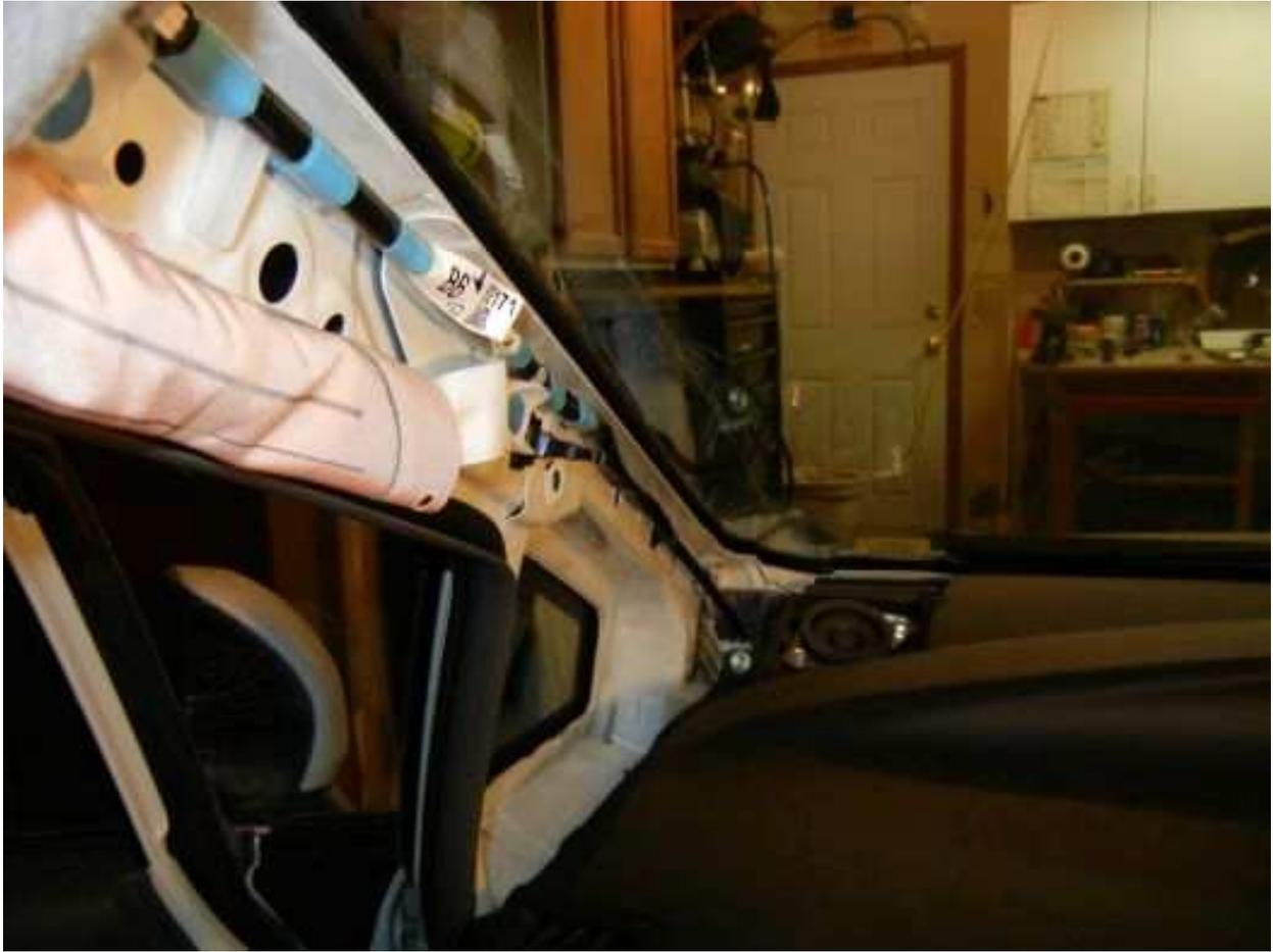
With the grills removed, use a 10mm socket to loosen the bolts holding the speakers in the dash.
