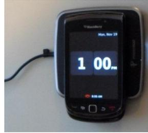
rubber holder and cut it apart to fit both the charger and the phone. My cutting was rather crude (I was in a hurry – it is getting cold here!) but I made a slot for the charger and a hole to allow the power cord to exit. I used 3M tape to hold the charger to the back of the holder and added extra 3M tape to the back of the holder to attach to the car.
