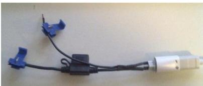
operation. It is by far the smallest one I have seen so I decided to use that. The picture does not give you a good idea of scale but it is only about 3" long by 1" square. I adapted the airplane plug and soldered on some wire leads and fuse to connect to a 12v source in the car.
