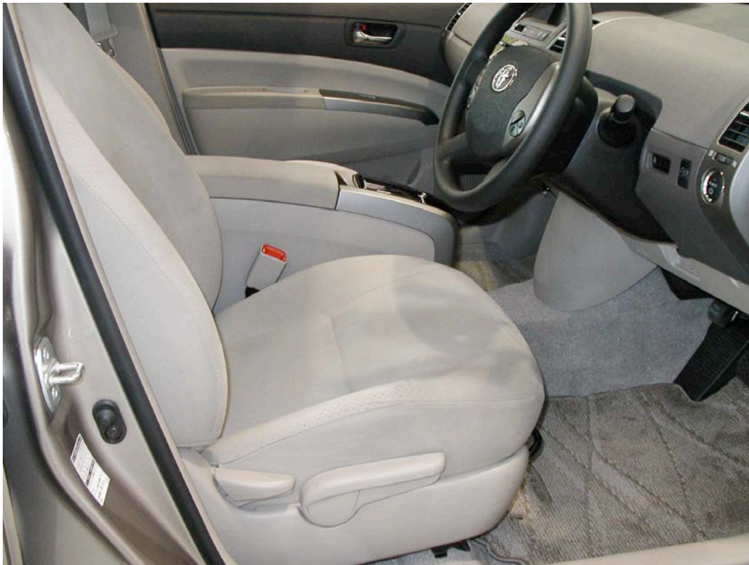
2006 Prius, Japan. Note “pump-handle” height-adjuster
