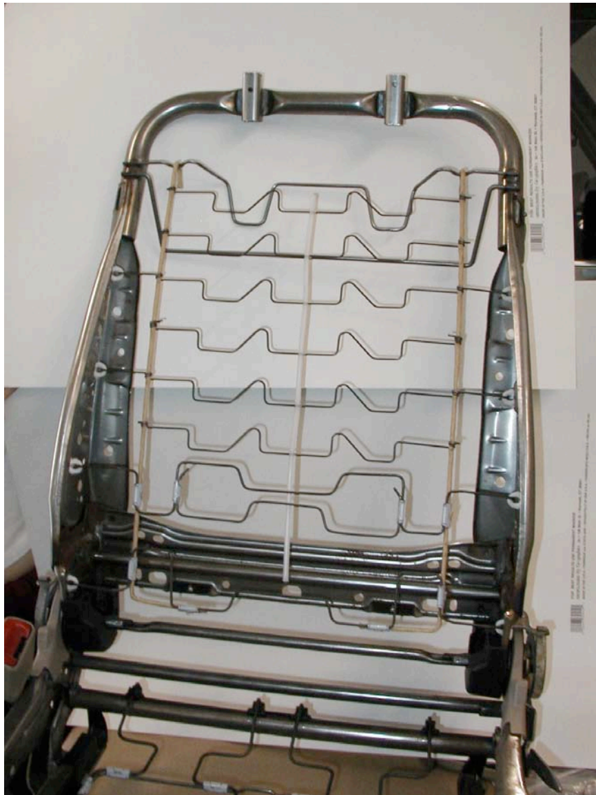
2005 Corolla Seat, stripped. Note, "squared" profile of seat top
