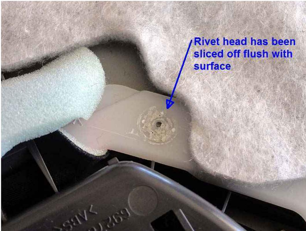
Rivet head has been sliced off flush with surface
