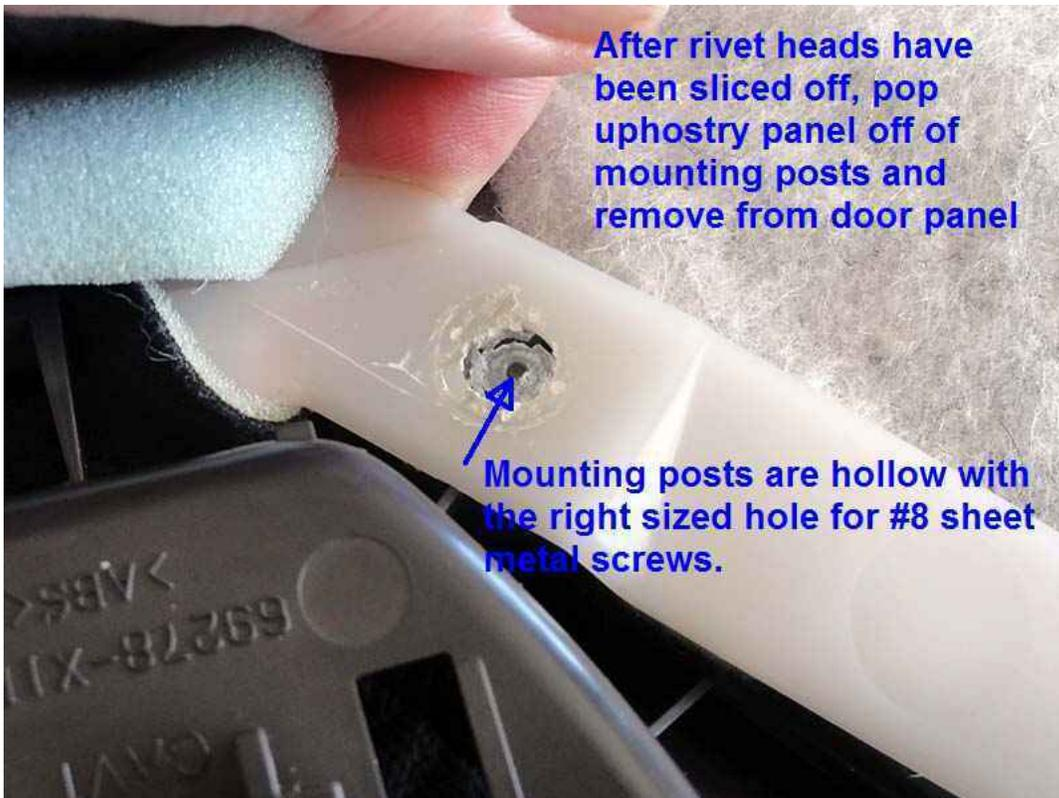
After rivet heads have been sliced off, pop upholstery panel off of mounting posts and remove from door panel
