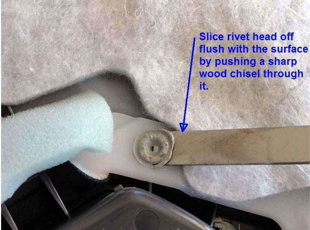
Slice rivet head off flush with the surface by pushing a sharp wood chisel through it.
