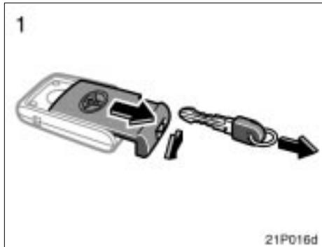
1. Remove the mechanical key and cover with slide the lock knob in the arrow direction.
