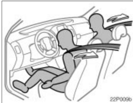
**There are seat belt pretensioners for both front seats. They are designed to be activated in response to a severe frontal impact.**
