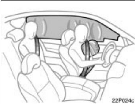
The SRS (Supplemental Restraint System) side airbags and curtain shield airbags are designed to provide further protection for the driver, front passenger and rear outboard passengers in addition to the primary safety protection provided by the seat belts.
