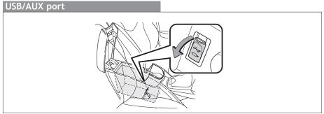
By inserting a mini plug into the USB/AUX port, you can listen to music from a portable audio device through the vehicle's speaker system while in USB/AUX mode.
