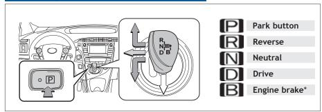
\* The engine brake is the equivalent of downshifting. Shift to "B" when engine braking is desired (i.e. downhill driving, coasting to a stop, etc.).
