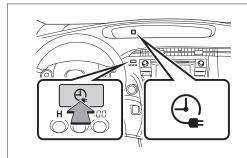
Once set, the time display will change from flashing to solid, and the charging timer indicator on the instrument cluster will come on.
