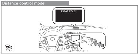
In distance control mode, vehicle will cruise at a set speed, decelerate to maintain selected distance from a slower vehicle traveling in front, and accelerate back up to the selected speed if the vehicle in front changes lanes or speeds up.
