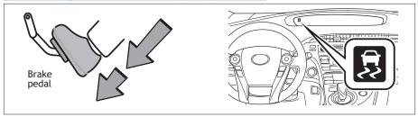
HAC helps prevent rolling backwards on an incline. To engage, push further down on brake pedal while at a complete stop until a beep sounds and slip indicator illuminates. HAC holds for approximately two seconds after releasing brake pedal.
