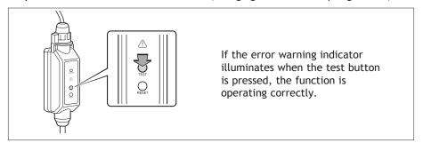
Step 3 Press the reset button on the CCID (Charging Circuit Interrupting Device).
