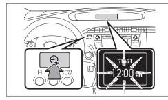
The timing display will change from solid to flashing.
