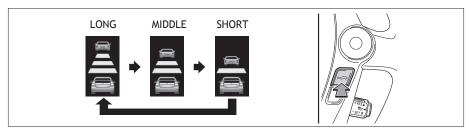
(3) To change the vehicle-to-vehicle distance Push the distance button to cycle through the settings, which will change progressively from LONG to MIDDLE to SHORT.
