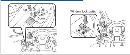
**Automatic operation** Push the switch completely down or pull it completely up and release to fully open or close. To stop the window partway, operate the switch in the opposite direction.
