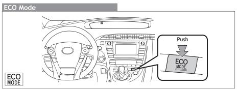
ECO Mode helps achieve low fuel consumption during trips that involve frequent accelerating and braking.
