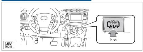
EV/HV Mode allows the electric motor (traction motor), powered by the hybrid battery (traction battery), to be used to drive the vehicle under certain driving conditions.
