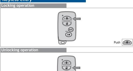
**NOTE:** If a door is not opened within 60 seconds of unlocking, all doors will relock for safety.
