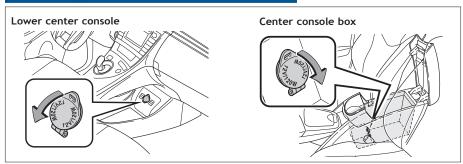
Power switch must be set at "ACCESSORY" or "ON" in order to use power outlets.
