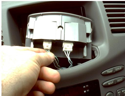
\_\_\_\_\_ 8. Remove two 10MM nuts now visible just below the screen.
