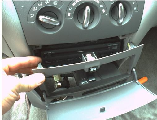
\_\_\_\_\_ 5. Unscrew the 2 Black Phillips screws near the upper corners of the CD player which are fasteners for the upper dash.
