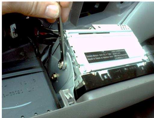
\_\_\_\_\_ 14. Lift straight up and out on the display screen to remove it from the dash panel.
