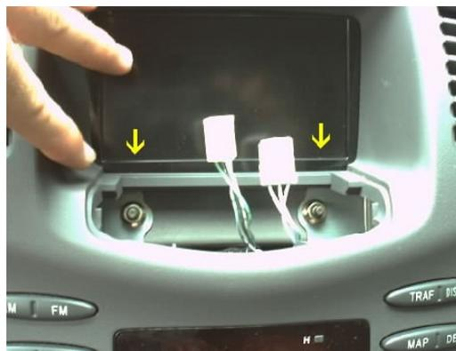
\_\_\_\_\_ 9. With the nuts out all you have to do is pull forward on the entire upper dash and it will release from the clips along the top edge (The clips are marked in the Photo below). You can also use a flat blade screwdriver to pop it outward if you need to. You only need to move it out a few inches to expose the display screen.
