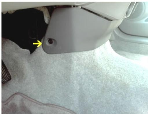
\_\_\_\_\_ 4. Open the door in the lower section of the dash covering your CD. Pull the bottom section of the dash outward and release it from the clips on the upper corners by carefully pulling outward or with a screwdriver along the top edge to help.
