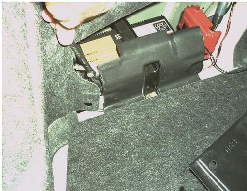
\_\_\_\_\_ 3. Back in the car, look below and to the side of the power outlet and notice the black plastic retainers on the corners on each side. Press in the centers of the retainers (same style as battery cover) on each side and remove them for reinstallation later.
