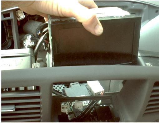
\_\_\_\_\_ 15. Thread the four 8MM bolts back into the holes in the display so that you won't lose them and lay the display aside.
