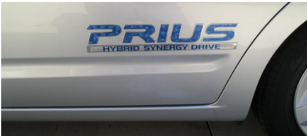
Picture 4: Stripe Tape Installed after Application Tape (Top Paper) Removed
