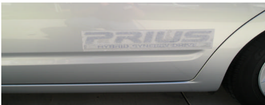
Picture 3: Stripe Tape Installed before Application Tape (Top Paper) Removed
