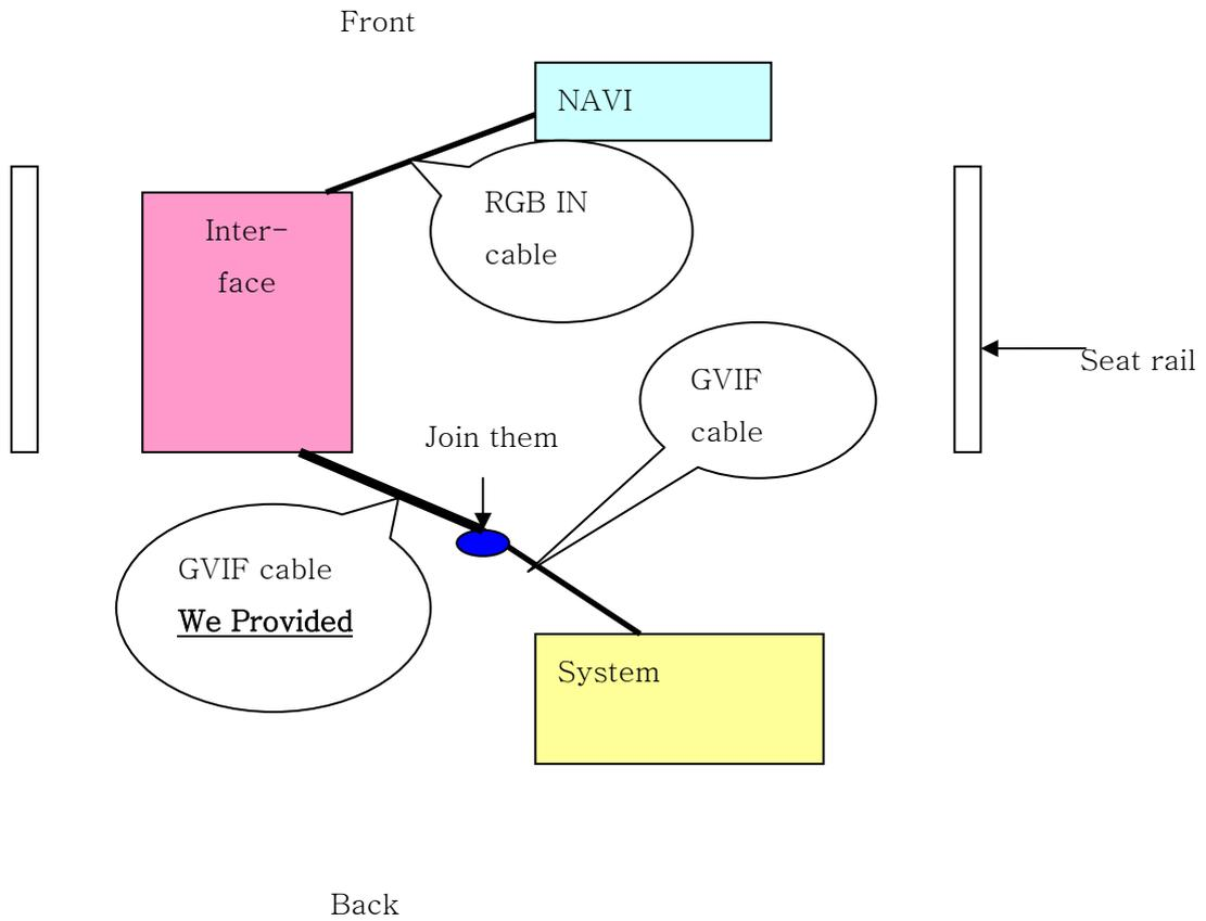
GVIF cable is located under the front seat.
