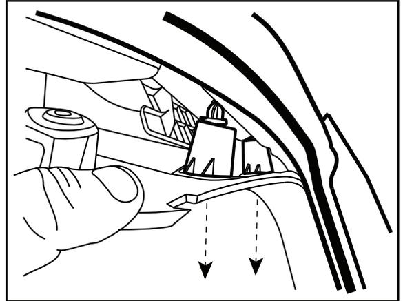
4. Hold the T-anchor stud and unscrew the T-anchor. Remove and discard the T-anchor and stud.
