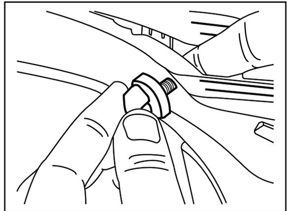
5. Snap the lower quarter panel trim back into place. Ensure that the weather strip is properly installed behind the tail light assembly.
