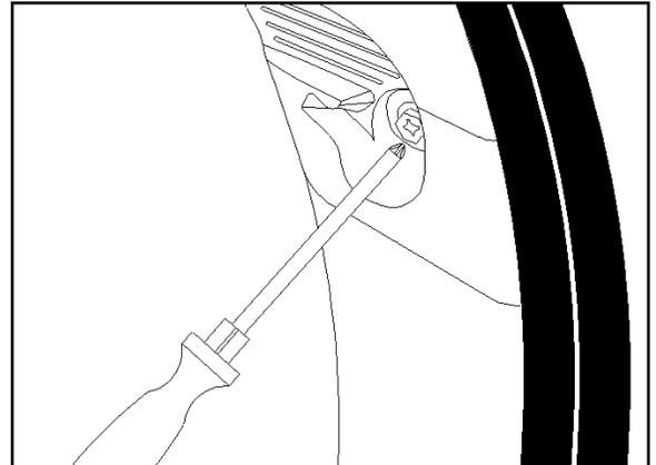
2. Using a plastic pry tool, disengage the lower quarter panel trim.
