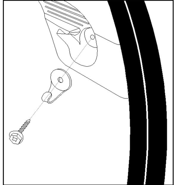
7. Plug the hole (from removal of the original T-anchor) in the panel with one of the plastic plugs in the repair kit.
