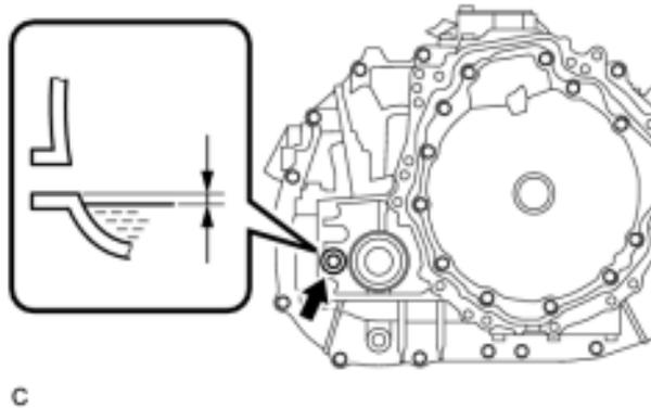
(b) Check for leaks if the quantity of transaxle fluid is low.
