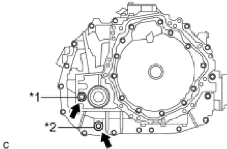
(b) Using a 10 mm hexagon socket wrench, remove the drain plug and gasket.
