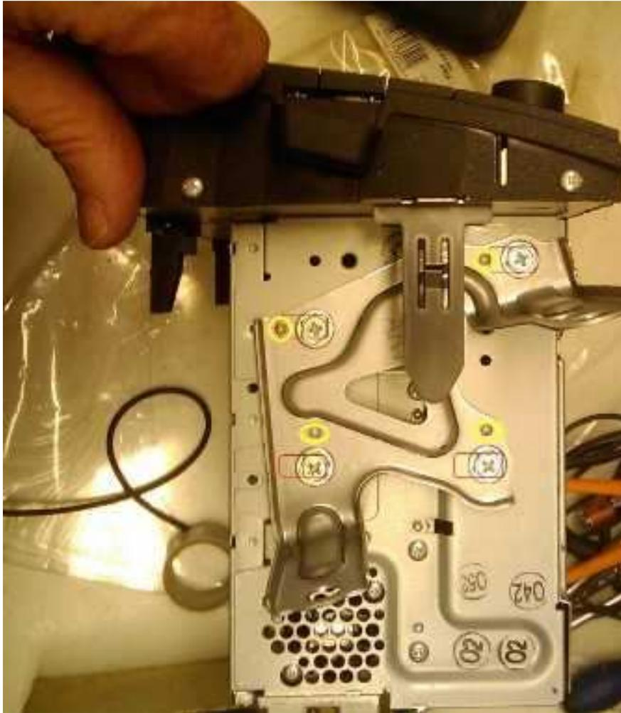
Note the yellow areas indicate dimples that have to be ground down as well. The red squares indicate the material that needs to be removed.
