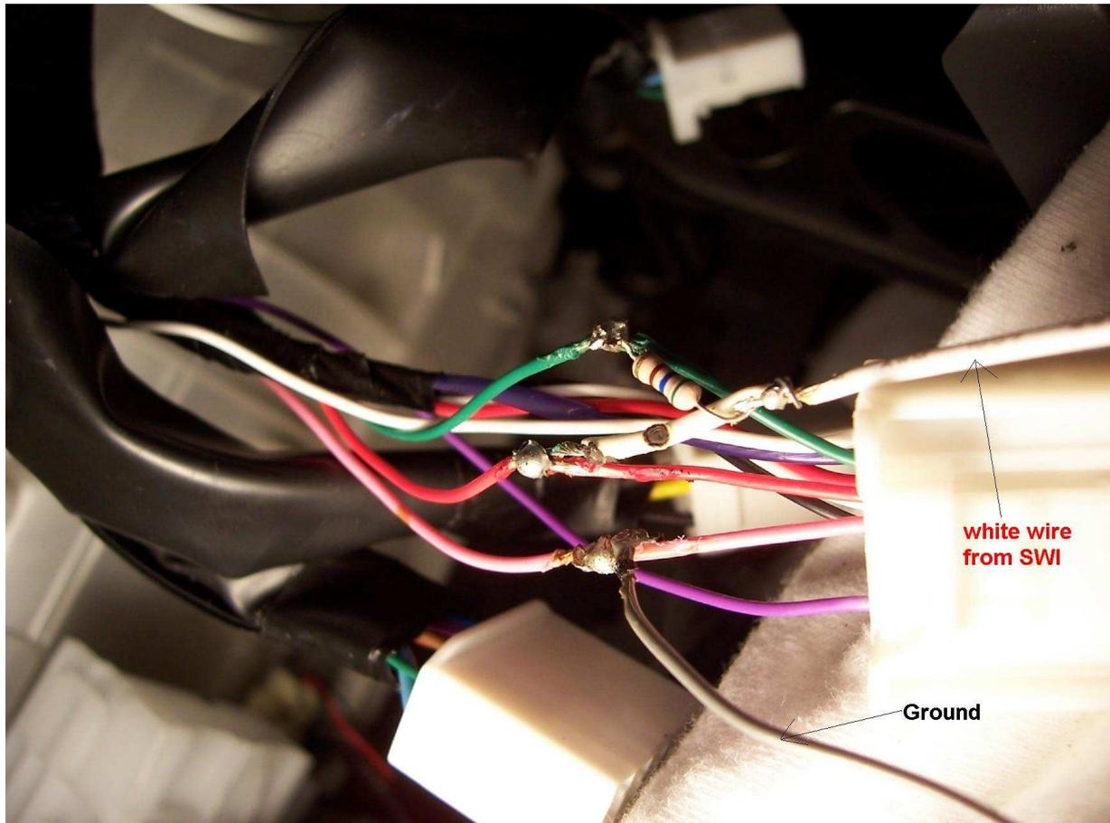
With the wiring harness connectors plugged in, you should be able to plug the power switch in and put the car in ACC mode. The head unit should activate and you should be able to confirm that it works properly.
