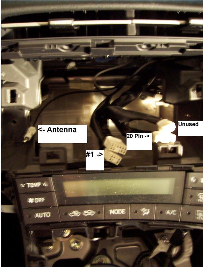
The following picture illustrates how I wired in the SWI to the car's wiring harness.
