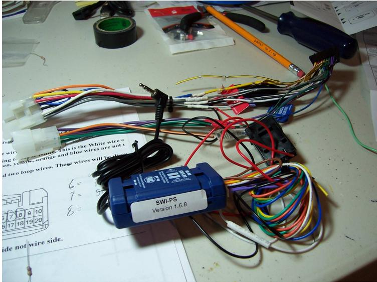
There will be a white wire from the SWI that will need to be connected directly to the car's wiring harness. See the "New head unit mounting" section below. All the other wires from the SWI can be wrapped up and tied off to reduce the mess.
