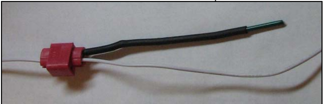
Connect resistor wire to white SWI-PS line with a tap-in connector.
