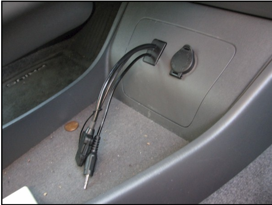
Option 2: Drill & slice the plug & run the cables through. (The butchered left side of the 'blank' plug isn't so pretty)
