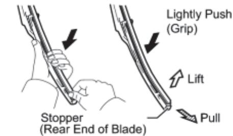
(a) Lift and pull the end of the wiper rubber protrusion from the blade stopper as shown in the illustration.
