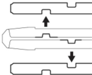
(b) Remove the 2 wiper rubber backing plates from the wiper rubber.
