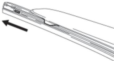
(a) Remove the wiper rubber with the wiper rubber backing plates from the front wiper blade.
