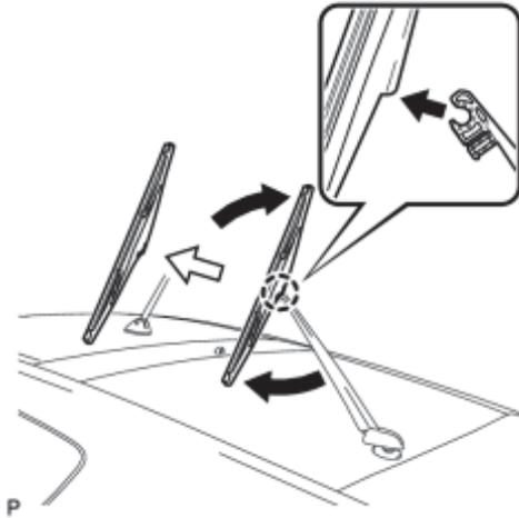
(a) Raise the wiper blade to the position where the claw detaches with a click sound as shown in the illustration.
