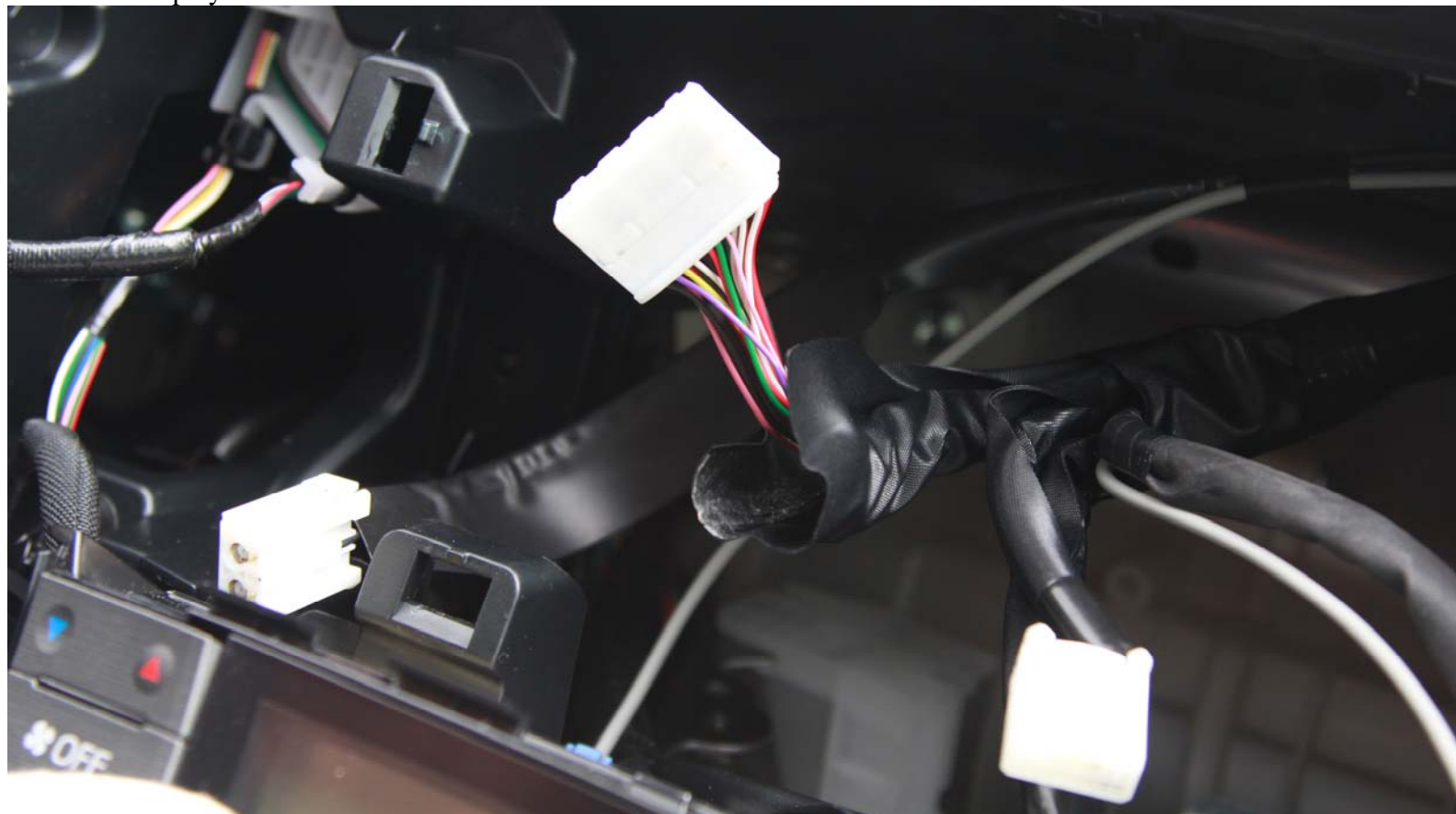
Unwrap the plastic wire cover and locate the Vehicle Speed Sense wire (violet wire) on pin 17.
