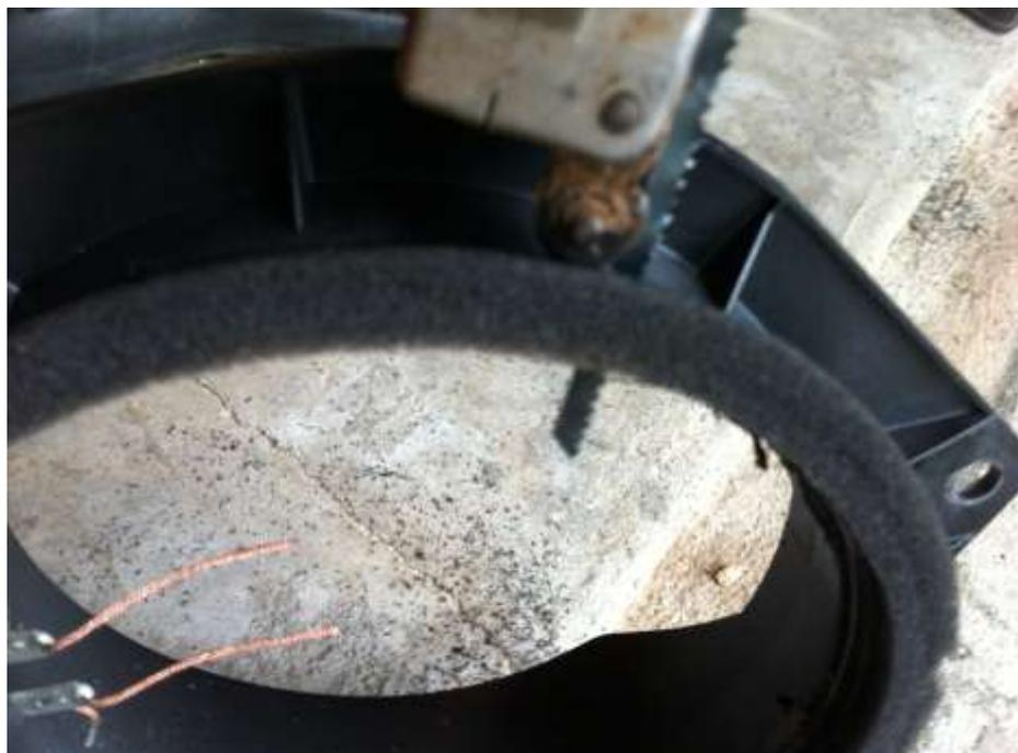
Bend the two enclosure contacts toward the back of the enclosure so they don't interfere with the contact board on the Polk. Then align the Polk's contact board with the enclosure contacts and check out how well it fits (like it was made to fit!).
