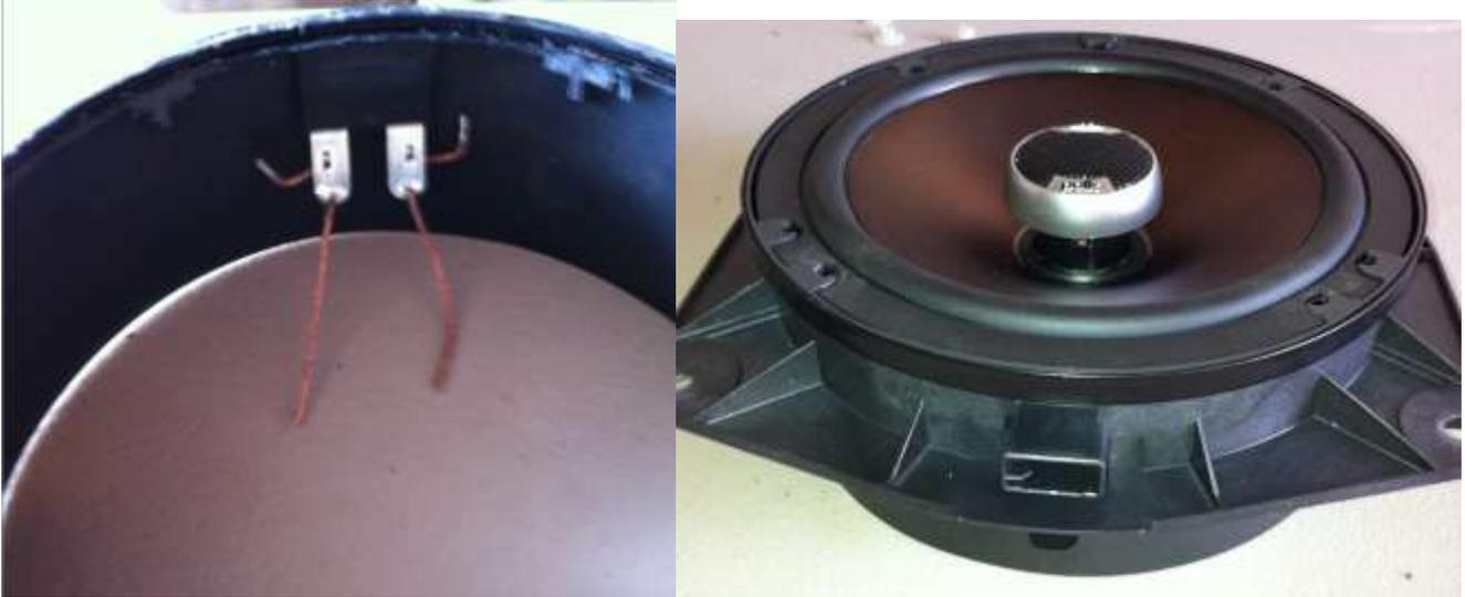
Here's where I had to get tricky with the wiring. I used an electrical meter to test which wire in the car is really positive. In our car, it's the white wire, and the red wire is negative. The Crutchfield wiring harness presumed the red was positive and white was negative. Who knows, maybe it's supposed to be. Anyway, I had to cross the contact wires over and use some electrical tape to prevent shorting. Don't let the solder drip on the speaker cone.
