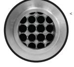
AFTFRMARKFT COMPETITOR 20 spiral tubes over cools exhaust gasses leading to increased soot production potentially causing premature . engine wear and downstream emissions problems
