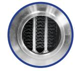
ORIGINAL EQUIPMENT Fin-and-tube design offers efficient thermal transfer but is more prone to soot clogging than tube-type cooler
