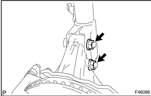
(b) Remove the 2 nuts on the lower side of the shock absorber.
