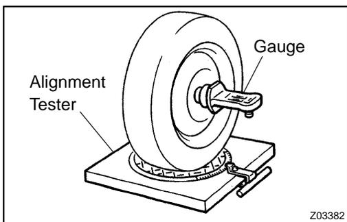
**6. INSPECT CAMBER, CASTER AND STEERING AXIS INCLINATION**
