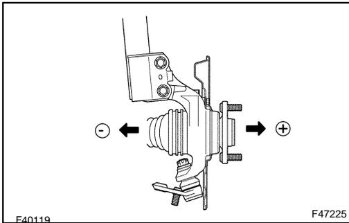
(e) Fully push or pull the front axle hub in the direction of the required adjustment.
