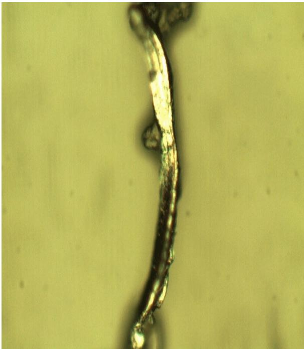
**Figure 1:** Ferrous Cutting Wear Particles and Abrasive/Dust/Dirt Particles at the Head of the Slide (Magnification 400X).
