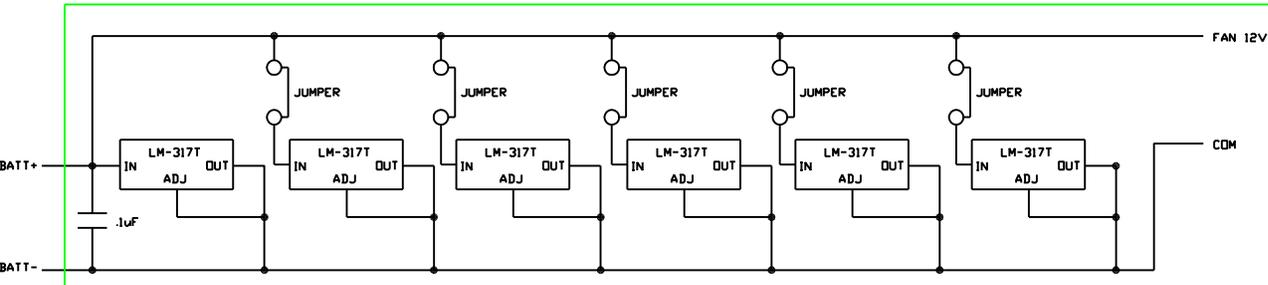
METAL TABS ON LM317'S CONNECTED THROUGH HEATSINK
