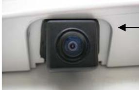
Camera mounted to the rear outer panel
