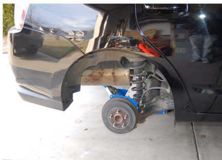
Step 1 - Removing the Wheels
