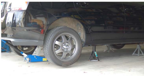
Step 1 - Removing the Wheels
