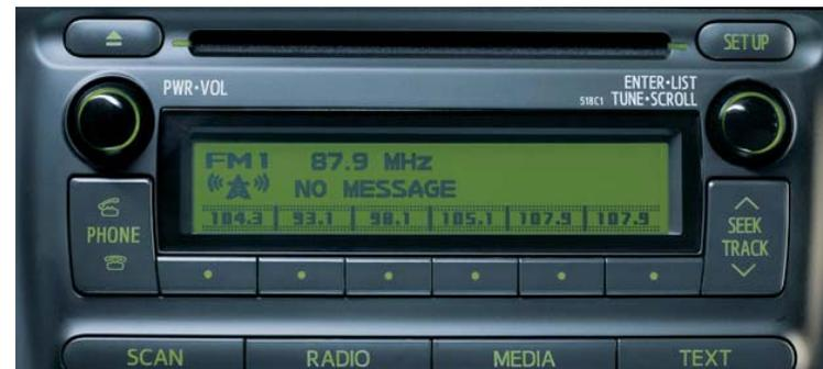
The standard audio system on Prius c delivers sweet sound at a sweet price. For starters, it's equipped with four speakers or available with six. And with a USB port, auxiliary audio jack and Bluetooth® wireless technology, the system provides you with hands-free phone capability, phone book access and music streaming.
