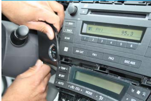
Step 5. Remove the trim around the push to start button
