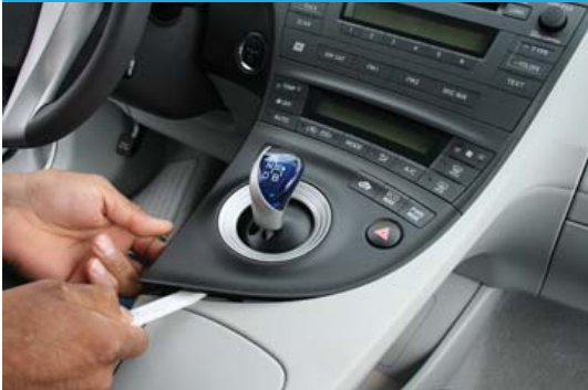
Step 4. Remove the trim from around the radio
