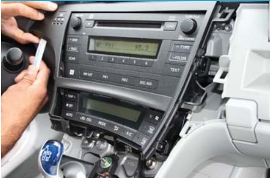
Step 4. Remove the trim from around the radio
