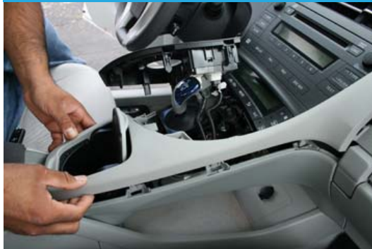
Step 5. Remove the trim around the push to start button
