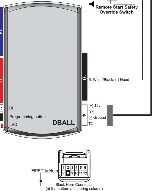
**!** See page 6 for help on locating key components in the vehicle and wiring reference chart.
