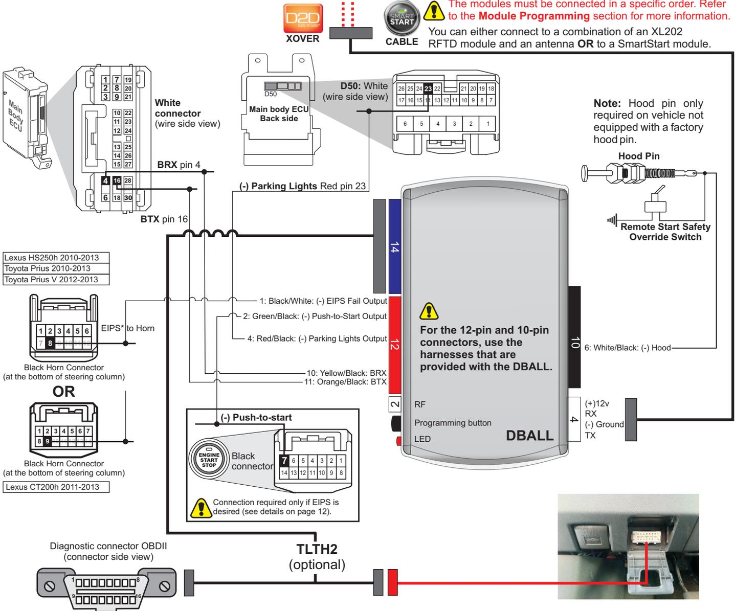
**Warning!** See page 12 for help on locating key components in the vehicle and wiring reference chart.
