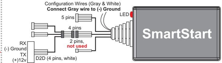
**Warning!** The modules must be connected in a specific order. Refer to the **Module Programming** section for more information. You can either connect to a combination of an XL202 RFTD module and an antenna **OR** to a SmartStart module.
