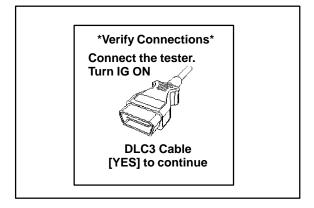
14. The Diagnostic Tester is currently confirming that the CAN Interface Module has been updated. If not, the next three screens will be displayed. If the CAN Interface Module has been updated, proceed to Step 18.
