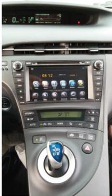
Now your radio is installed. Finish up the routing of the GPS antenna, iPhone cable, and external usb extension cable from passenger side floor to the desired locations.
