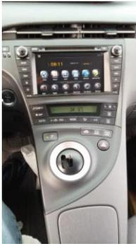
Install the trim around the shifter on. Note: I didnt notice till now that you do not have to remove the shifter knob to remove the trim around it (mine is missing from picture).Make sure all the trim is pushed in/down all the way around flush.
