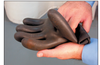
Figure 1 – A pair of rubber insulating lineman's gloves used when working around the high-voltage system parts is being rolled up to check for pinholes before using them.
