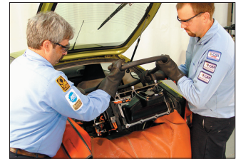
Figure 3 – The high-voltage battery on a 2001 Honda Insight is being removed using Honda's special battery removal tool.
