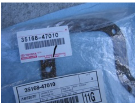
Use new pan gasket, around $12 at dealer part number 35168-47010
