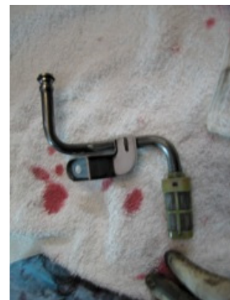
It is very important to clean input screen of the oil pickup tube. You can do this with pickup tube in car. Often the screen is plugged with gunk and after wiping fluid comes out...signifying poor ATF circulation due to plugged screen. If it gets too plugged you'll cook the tranny.
