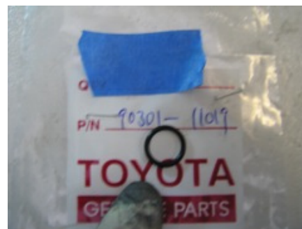
O-ring seal on internal pickup tube. Not usually necessary to remove the pickup tube but if you want to the part number for O-ring is 90301-11019.
