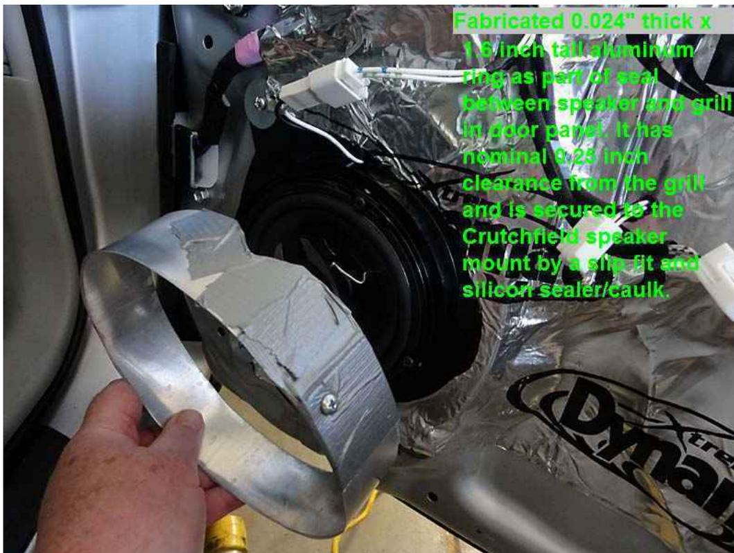
Fabricated 0.024" thick x 1/8 inch tall aluminum ring as part of seal between speaker and grill in door panel. It has nominal 0.25 inch clearance from the grill and is secured to the Crutchfield speaker mount by a slip fit and silicon sealer/caulk.
