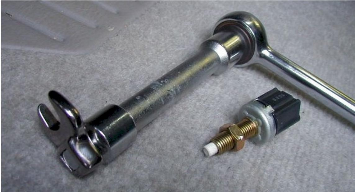
After getting the wrench on the nut and holding it in place with one hand, I thought carefully about which way to turn (clockwise) and gave a good tug on the driver with the other. I felt the nut turn and the switch then unscrewed by hand. Maybe I was lucky. There are discussion group posts that make getting at that nut look *much* more difficult than I found it. If you have trouble, I think a proper 3/8 inch drive would work even better than my clunky 1/2 inch drive and adapter.
