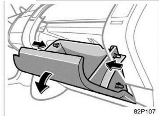
4. Push in each side of the glove box to disconnect the claws.
