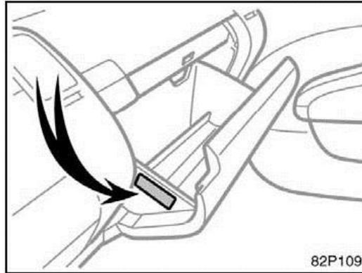
The air conditioning filter information label is placed on the left side of the glove box as shown and indicates that a filter has been installed.
