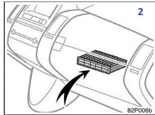
The air conditioning filter is set behind the glove box.
