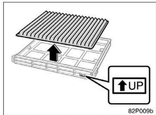
6. Remove the filter from the filter case and replace it with a new one.
