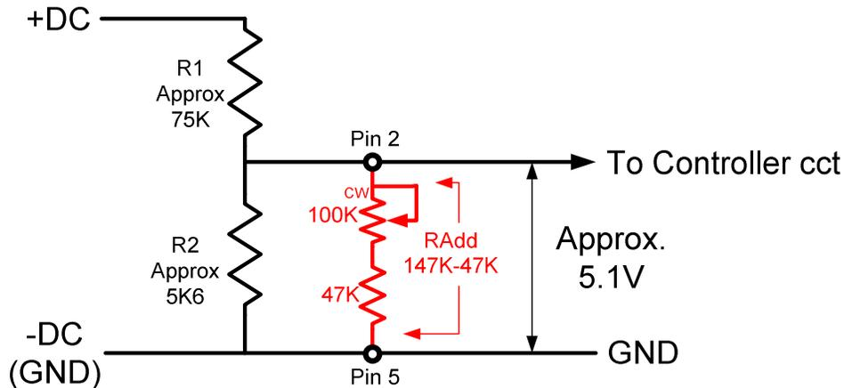
So all we need to do is add a parallel resistance ( $R_{Add}$ ) across the  $R_2$  (5K6) between Pin 2 to Pin 5 and we can change the divide ratio. I did this with a 47K resistor and 100K pot shown in **red** above.
