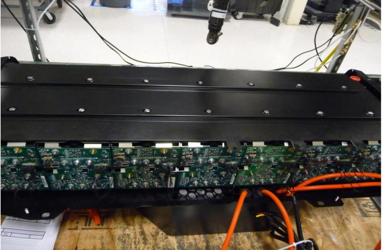
**NOTE: Even with the MSD disconnected, each half of the pack (3 and 4 modules connected in series) has a potential of roughly 80 and 100 Volts from end to end, respectively.**
