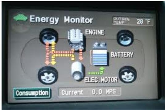
when your battery is failing it will not accept very much energy from charging system. This will cause the SOC to turn green even though the battery has little energy in it. Sometimes people forget that when new the SOC display rarely or never showed green bars on the SOC or displayed it fully charged. A healthy battery will not turn green very often, if at all. It is normal to show about 2/3 to 3/4 full when driving at steady state speeds not using the hybrid system.
