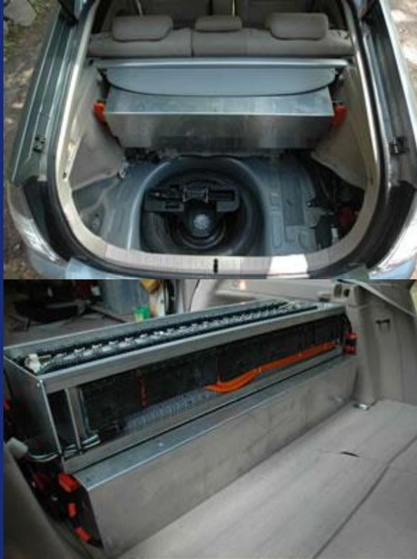
It is also possible to rearrange modules to use the space where the spare wheel went for some of the modules such that enough space then exists above that (but still under floor) for the other modules plus the charger so that nothing is normally visible:
