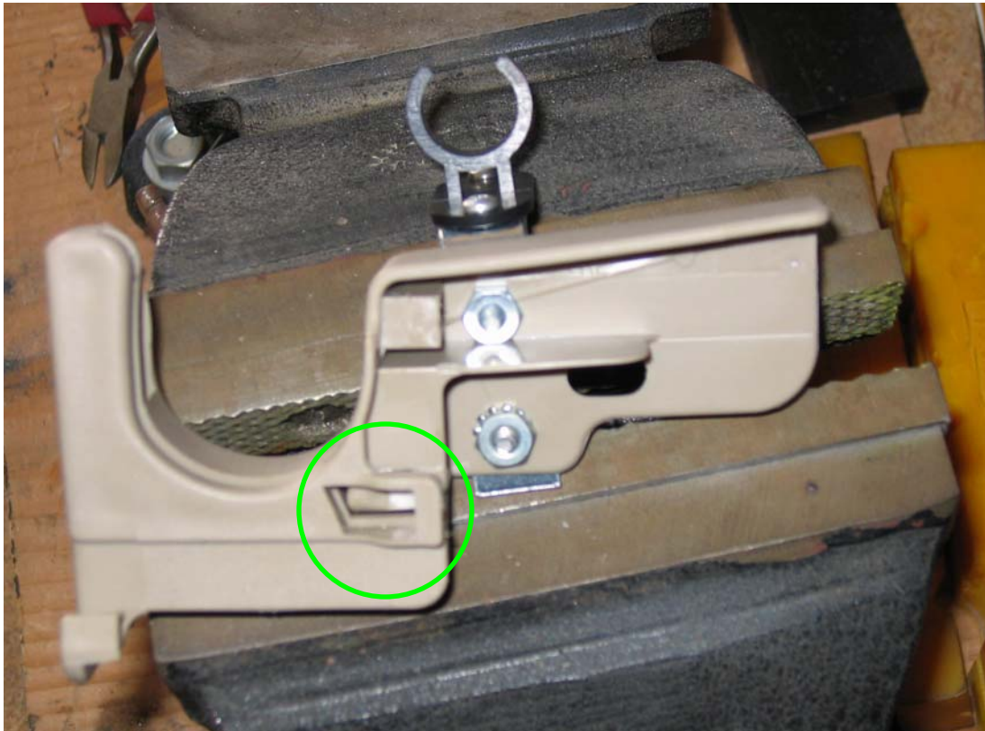
Back side view of the seat rail cover. Plastic catch is circled in green.
