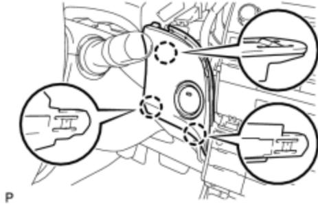
(b) Disconnect the connector and remove the upper instrument panel finish panel sub-assembly.
