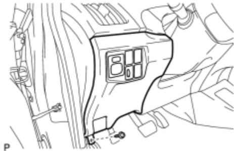
(a) Remove the screw <C>.
