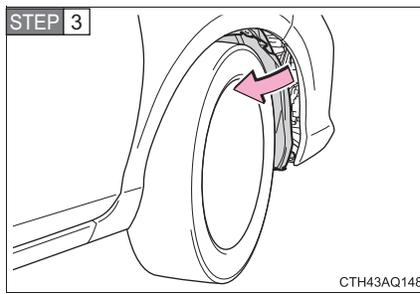
Partly remove the fender liner.
