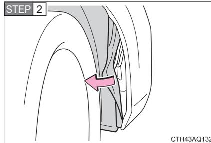
Partly remove the fender liner.
