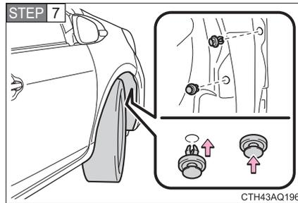
Installing the clips.
