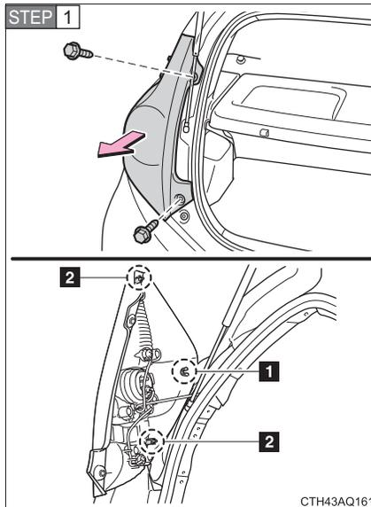
Open the back door and remove the bolts. Pull the lamp assembly straight back to disengage the clip and 2 pins.
