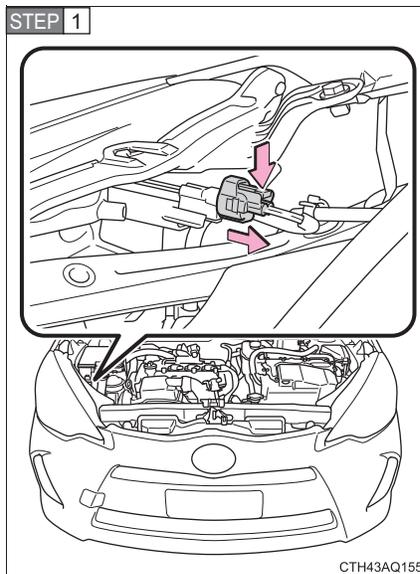
Unplug the connector while pushing the lock release.
