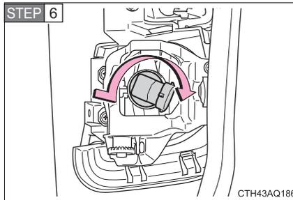
Turn and secure the bulb. Install the connector.
