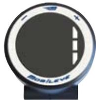
Headway Monitoring assists the driver in keeping a safe driving distance, and issues an alert when the headway distance becomes dangerous.
