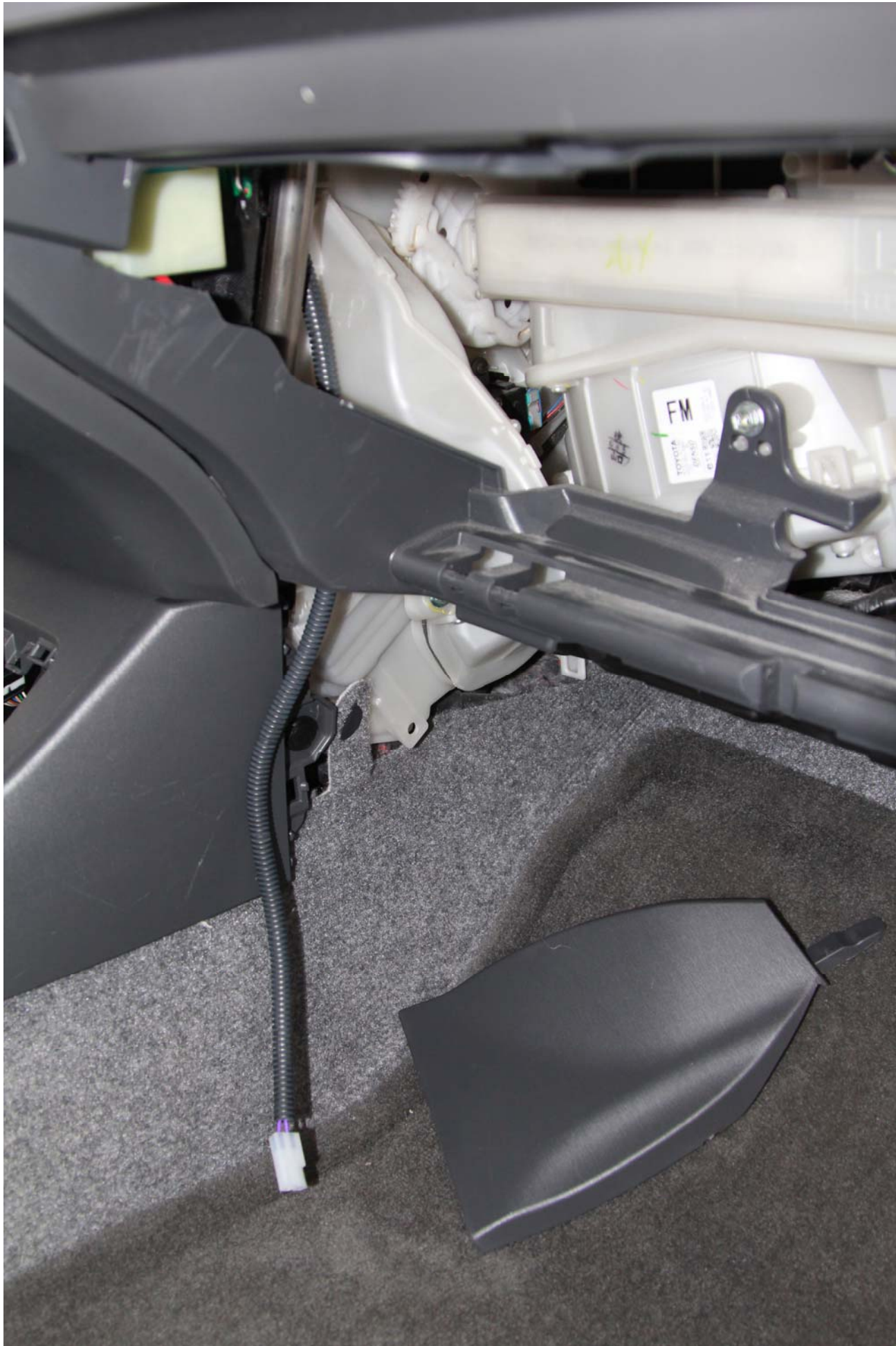
Route the VSS extension harness to the lower center console.
