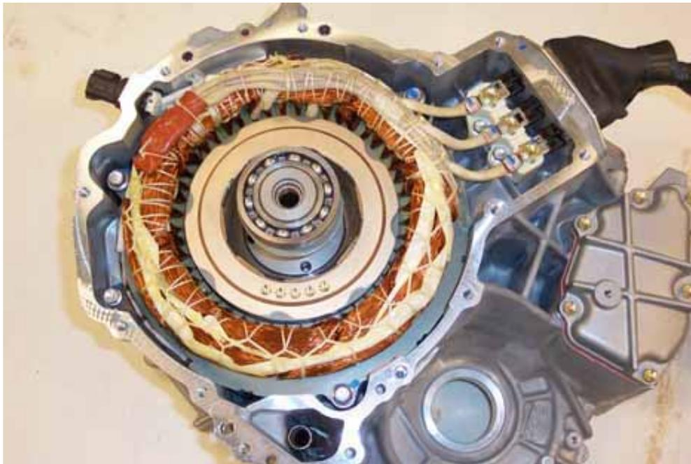
Fig. 2.8. 2004 Prius motor rotor and stator.
