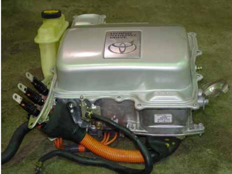
**Fig. 2.9. 2004 Prius inverter and converter unit.**
