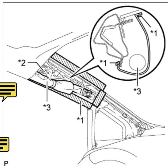
**28. DEPOSER LA PIECE DE COIN DU GARNISSAGE DE MONTANT AVANT GAUCHE**
