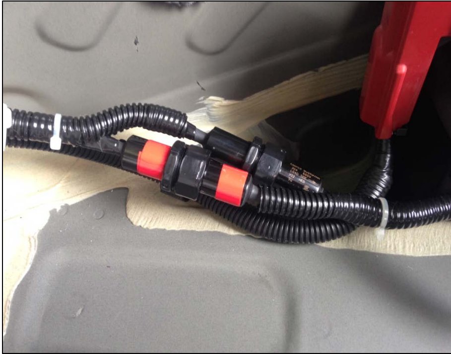
Figure 5 - Close up of the fuses split out of the wiring loom. The positive (+) wire is marked with red electrical tape.
