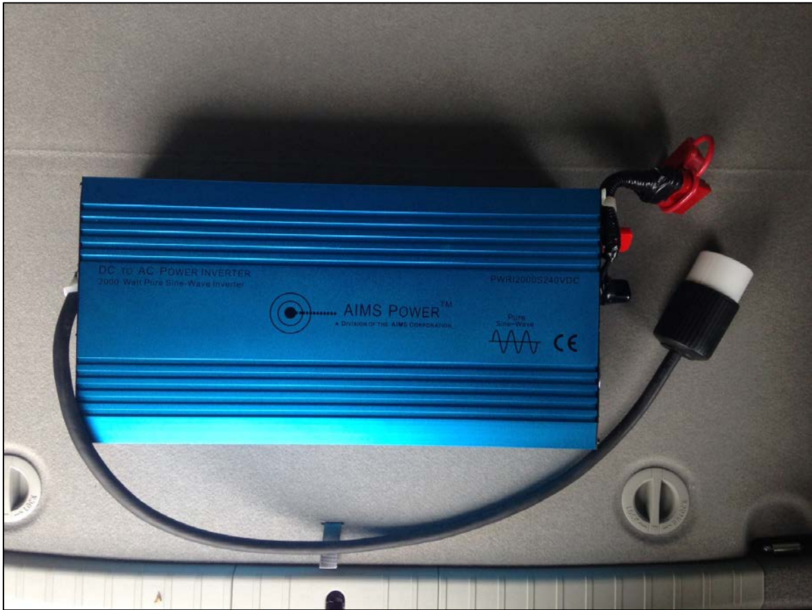
Figure 10 - Inverter with red Anderson connector on the 240VDC input side (right) and the cable for connecting the 120VAC side to the transfer switch (left).
