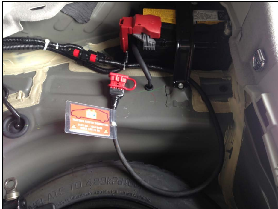
Figure 4 - Business end of the traction battery connection with the rear floor panels removed. Note the fuses (red stripe), capped Anderson connector and warning label. The 12V auxiliary battery is at the top right of the picture with the rear of the car to the right.
