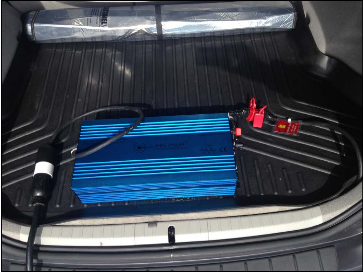
Figure 11 - A little difficult to see, but here is the inverter in use. The cable from the battery comes up from the lower right side of the picture and connects to the inverter. The inverter output on the left is connected to the cable that feeds the transfer switch.
