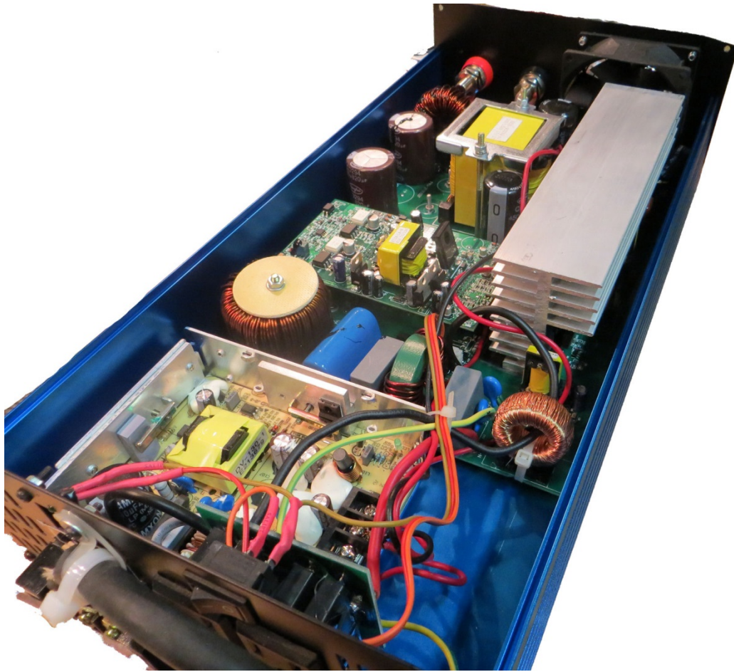
Figure 15 - Here's the interior of the inverter. Nice build quality by AIMS.
