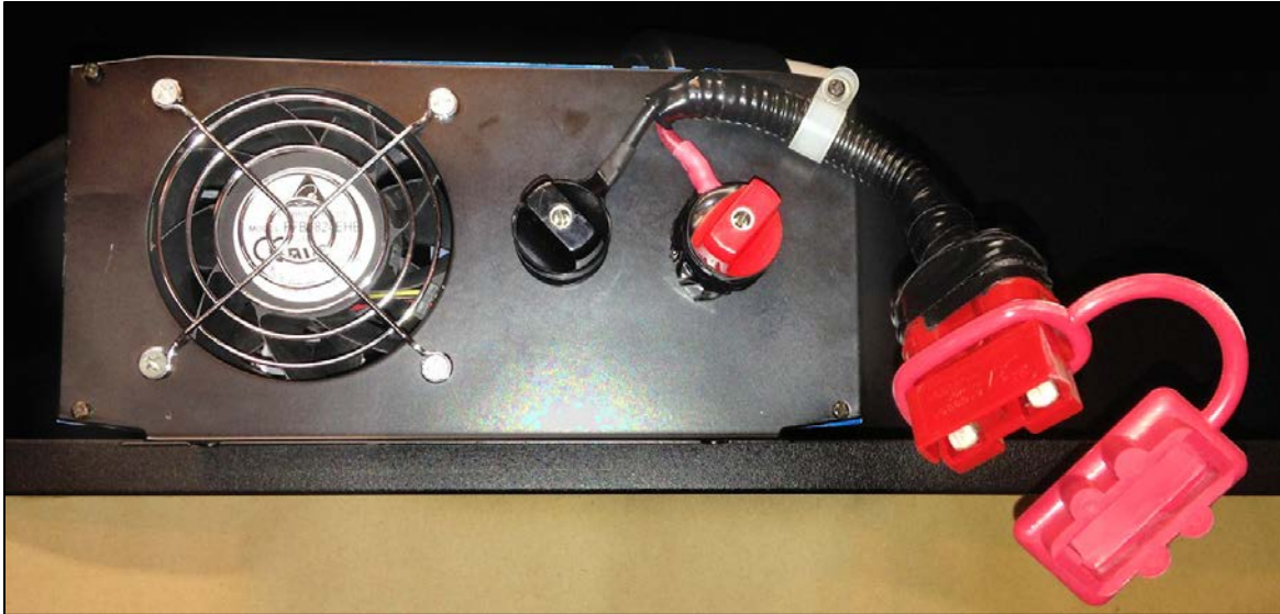
Figure 9 – The 240V DC input side of the inverter. Note the strain relief, wiring loom, taped thumbscrew terminals and taped Anderson connector. In the future, I will probably drill a hole in the end plate and make the connections inside the unit rather than using the thumbscrews/ring connectors.
