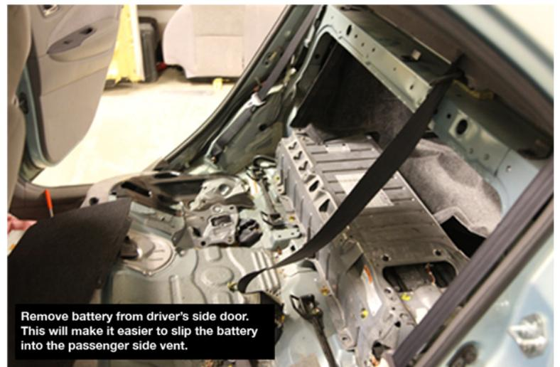
Replace switch last after new battery install. Replace carpet, seat cushions and then reconnect 12V negative cable.
