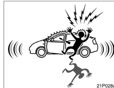
**To deter vehicle theft, the system is designed to sound an alarm if any of the doors or hood is forcibly unlocked or the battery terminal is reconnected when the vehicle is locked.**
