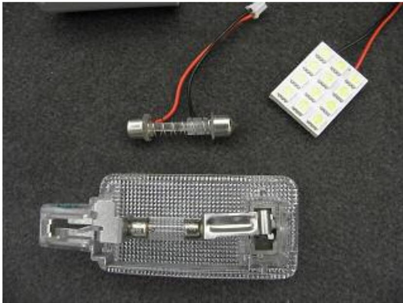
Next step is to connect the LED panel to the bulb connector, saving the plastic connector for use with the LED strip later.
