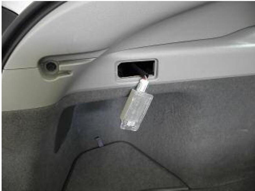
Un-clip the wire (releasing tab) and remove the rear grey plastic. Picture below shows the parts next to the disassembled light.
