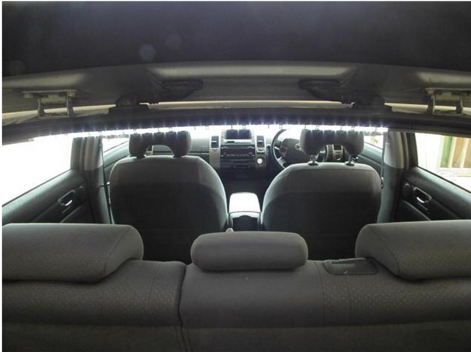
Next, I used the LED wedge bulbs in the front roof driver / passenger lights. This was very simple remove the old bulb, put in the LED & Test (swap the LED round if it does not work!)
