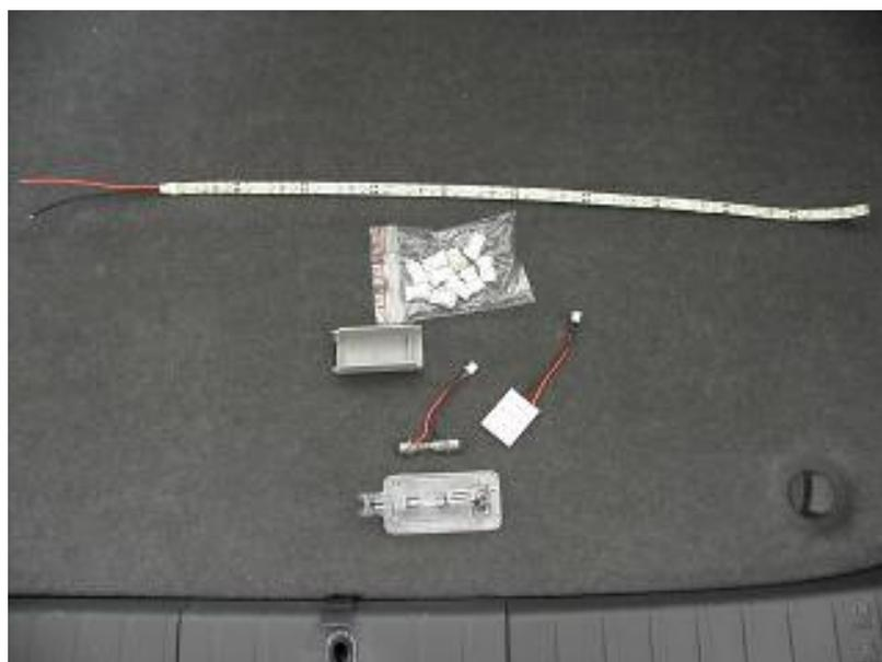
Close-up of the parts to replace the boot light:
