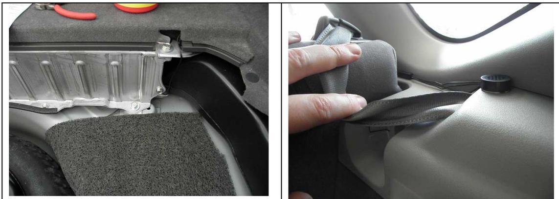
Next, stick the antenna onto the inside of the bumper and secure the ends with some of the included adhesive strip.
