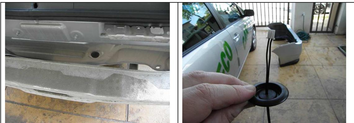
I located the electronics box near to the rubber plug in the spare tyre well to give me the maximum amount of length for the antenna wire. I also used the nearby grounding point (the bolt slightly left of centre in the photo) for the earth connection.
