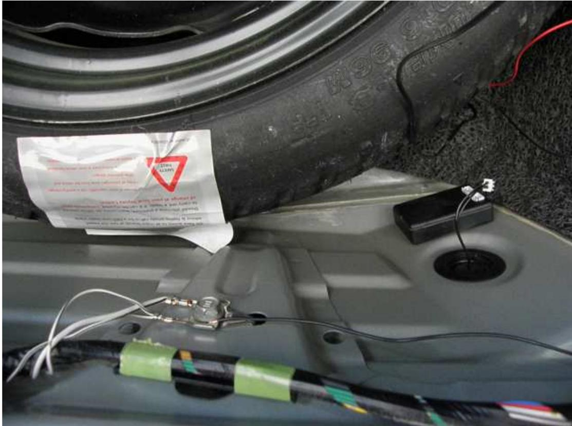
Tap into the +ve wire (purple/red on my car) on the reversing light above the 12v battery (I stripped the reversing wire and soldered the PD1 supply wire (red) onto it and covered with insulating tape and tie wrapped together)
