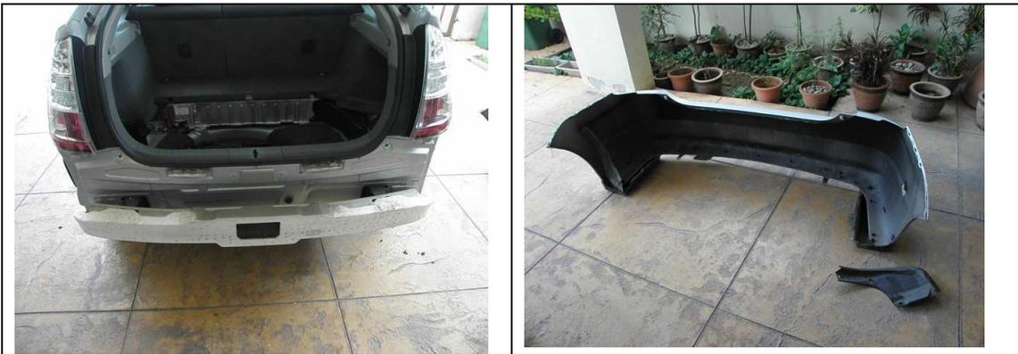
Wash the inner side of the bumper and allow to dry so that the sensor tape will stick to the interior of the bumper.
