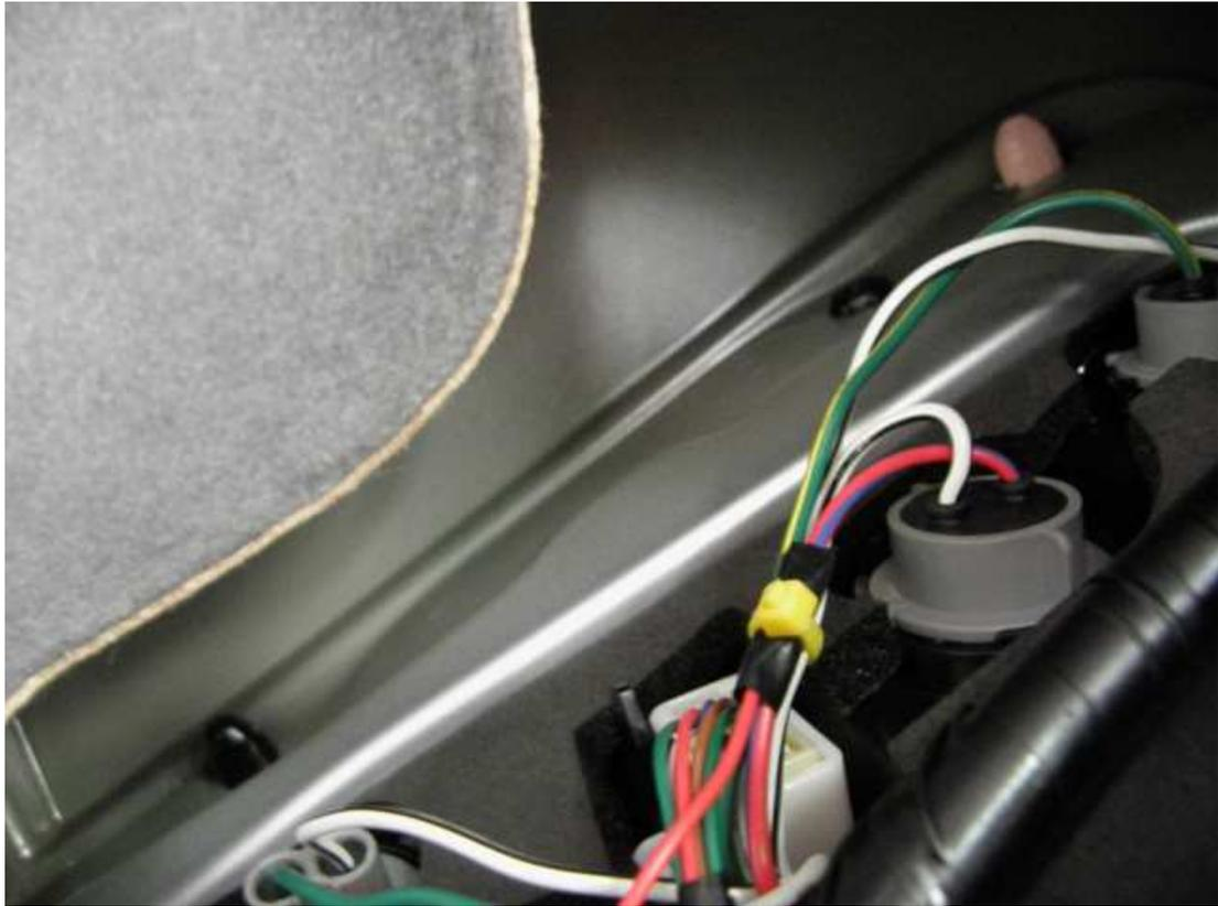
Next I routed the speaker wire to the shelf above the rear passenger seat, underneath the trim above the HV battery.
