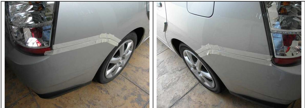
Using a very thin screwdriver covered in paper-tape to protect the paint, pop off the side panels. Use the screwdriver to push down the black lug which will release the panel.
