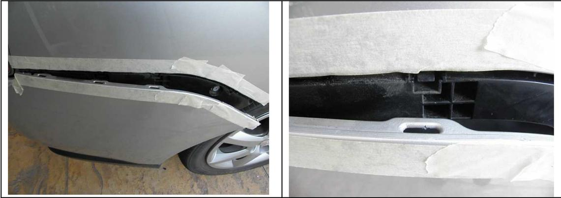
Remove the screws and fasteners from underneath the car and in the wheel wells.
